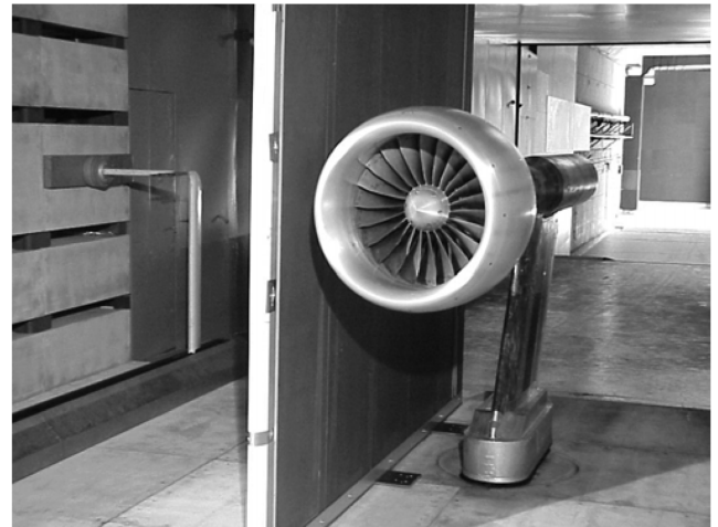
Fig. 3 Photograph of the research fan with the acoustic barrier wall in place.
